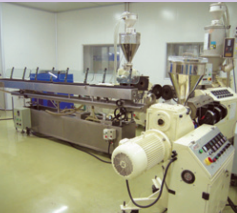
Cleanroom tubing extrusion capabilities
